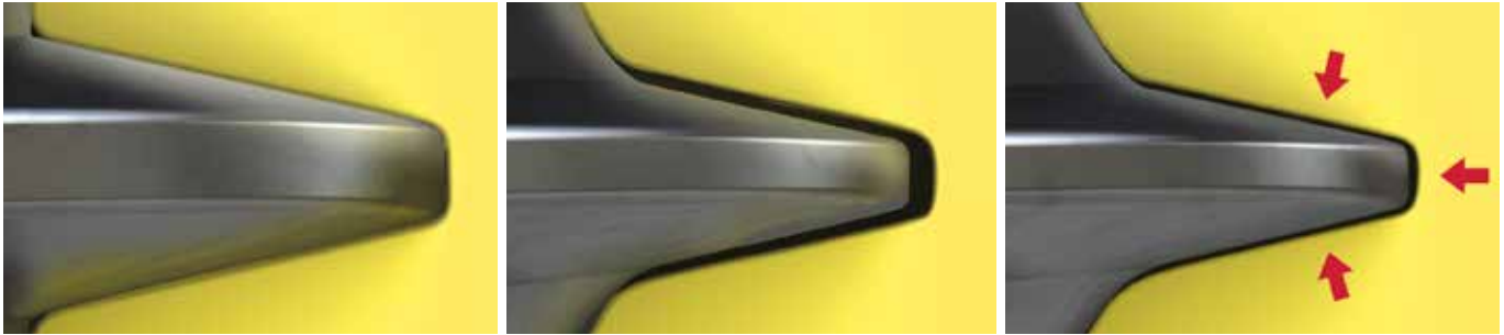
Thread forming zone forms thread turn into the material
