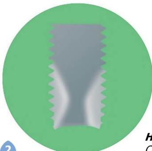
**CORFLEX®-‘N’ Heat Treatment** - CORFLEX®-‘N’ TAPTITE 2000® fasteners are neutral hardened to grade 10.9 strength level. CORFLEX®-‘N’ products are designed to be used in “soft white” metals such as aluminum or zinc alloys. CORFLEX®-‘N’ heat treatment can be specified for any size TAPTITE 2000® screws or bolts that are intended to be used in aluminum or zinc alloys.
