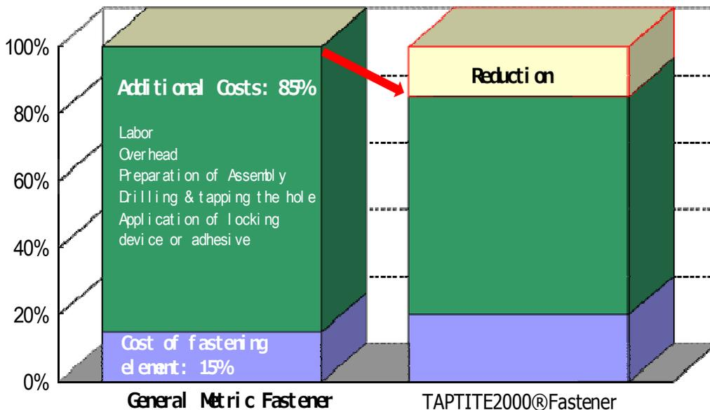
This chart shows a 10% increase in additional (assembly) costs results in an 8.5% increase in overall joint cost.
